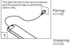
The receiver can store up to 3 sets of pairing codes. When a fourth remote control is paired, it will automatically cover the first one.
