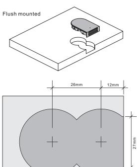
Use a 35mm drill to make holes according to the size shown above.
