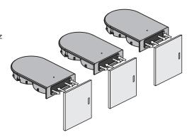
3 sensors can be used in combination. Open any door and the light will turn on.
